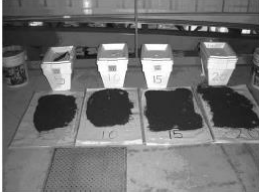
Figure 18-13. Styrofoam boxes labeled 5, 10, 15 and 20 minutes to measure the effect of post cooking time at 4 MT/hr.
