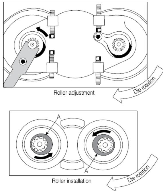
The rolls should be adjusted to allow a minimum clearance of approximately 0.051 cm between the
