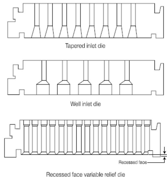
Die blanks are normally limited to a maximum of 12 cm overall thickness, so if the user is producing 19.05 mm or 25.4 mm diameter pellets, sometimes referred to as “cubes,” it is not possible to achieve the correct L/d ratio to produce a good quality pellet or cube. This is why a pre-compression chamber is necessary for these particular applications. These types of dies are used to produce good-quality cattle or sow cubes, and for use with high-fiber, light bulk density materials.
