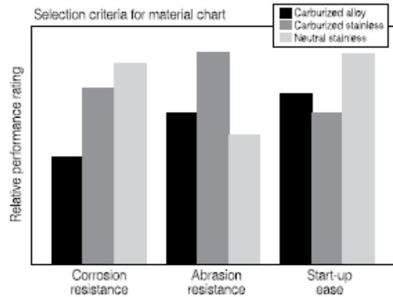
Case carburized alloy dies are usually the most breakage resistant and best suited for heavy tramp metal situations. They are used in heavily-abrasive situations, such as high mineral feeds, where die life with other materials is much shorter, keeping cost-per-tonne ratios to a minimum. They are the lowest-priced dies available when compared to the stainless steel dies. Alloy is most commonly used for the large-hole or “cube” dies. They should not be used in corrosive applications.
