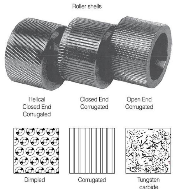
Dimpled shells have a series of specially-designed holes machined into the roller face surface. These shells are available with a shallow or a deep dimple, depending on the application. They have excellent wear characteristics due to the increased surface area of metal as compared to the corrugated shell.
