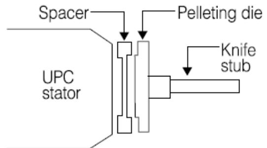
As the pellet leaves the die, a variable-speed rotary cutter controls the pellet length. For example, by increasing the cutter speed, short pellets and
