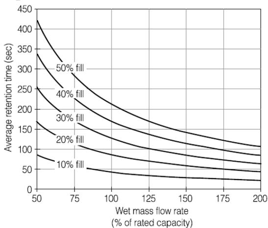
The fill factor will vary from 5% to 50% depending on the beater configuration, shaft speed and throughput. It is intuitive that configuring additional beaters to convey in a reverse direction will cause additional fill in the preconditioner. Conversely, configuring so that they convey in a forward direction will result in the opposite effect. From **Figure 2-5**, we can see that increasing the
