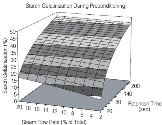
A well-designed and properly-operated preconditioner is capable of routinely cooking from 30-40% of the starch present in a given formulation, and under certain situations the cook level can approach 70%. A study was conducted in which the retention time and steam addition level were varied and percent starch gelatinization was measured as a response. The results of the study (Figure 2-8) indicate that increased retention time results in
